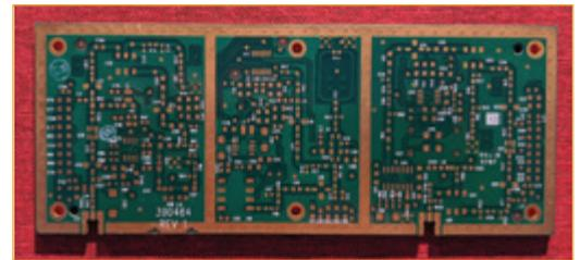
**FIGURE 2.** The thicker RF traces are required to accommodate test points without impedance issues. Traces can be thick only if the reference plane is a few layers deeper into the board.
