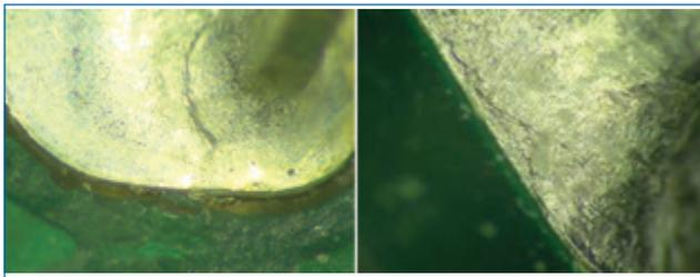
**FIGURE 3.** Optical images of cracks in the surface of low-temperature solder through-hole joints after thermal cycling. These cracks are located on the joint surface directly above the barrel of the plated through-hole at the solder fillet interface.
