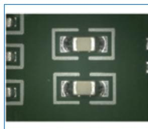
FIGURE 7. Component 0805 – after cleaning.
