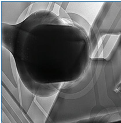
**FIGURE 5.** Magnified oblique angled x-ray image of low-temperature solder joint after 2,000 thermal cycles showing cracking all around the joint.
