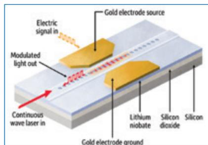
of 17.5GHz, switching speeds of up to 11Gb/s and a tuning efficiency of up to 1.98GHz/V. Applications include communications, computing, and quantum photonic information processing. (IEEC file #11886, *Laser Focus World*, 8/27/20)
