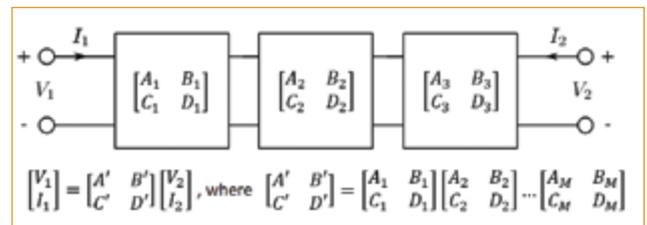
**FIGURE 1.** Cascaded ABCD network definition. The equation shows a cascaded matrix with M 2-port networks.
