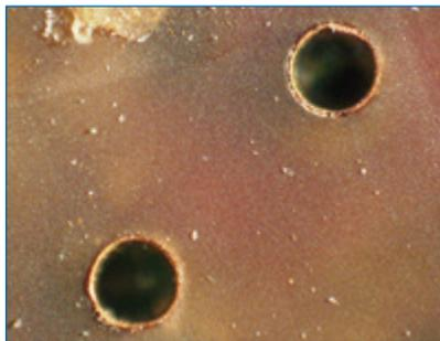
**FIGURE 2.** Post-separation, the inner-layer surface shows no visible adhesion.
