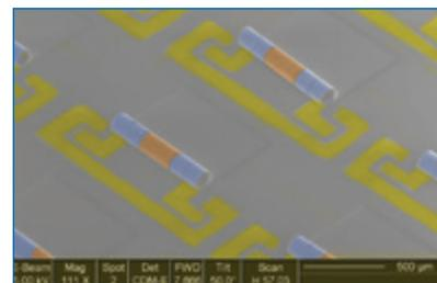
array of new chip components that combine the inductors (blue) and capacitors (yellow) needed to make electronic signal filters in phones and other wireless devices. (IEEC file #11865, *Microwave & RF*, 8/25/20)
