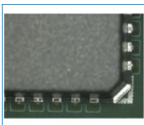
FIGURE 8. MLF-68 fully cleaned surface.
