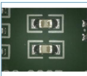
FIGURE 6. Component 0805 – before cleaning.
