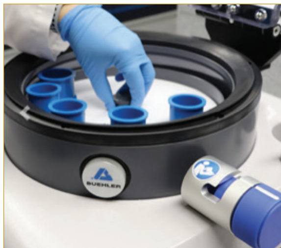
FIGURE 9. Vacuum system loading reduces processing time.
