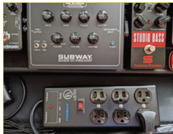
FIGURE 1. My Blackboard with a new surge protector that also filters EMI and RFI.
