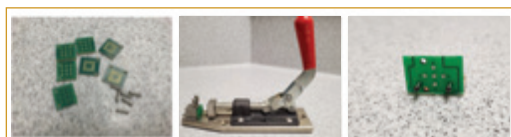
FIGURE 6. Coupons are loaded onto the pins using the pin locator.
