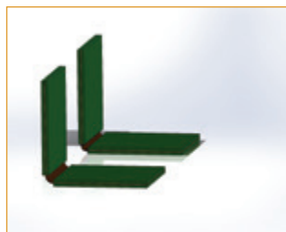
FIGURE 1. Adding strain relief can cause a much tighter bend radius on a short flex section.
