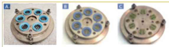
FIGURE 8. Coupons mounted into holder before pouring the resin (a), cured mounts in the mounting assembly (b), and the grinding fixture with the molding plate removed (c).
