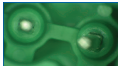
FIGURE 1. Connector pins that "float down" too far can damage soldering equipment.
