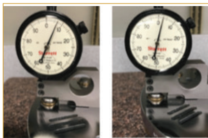
FIGURE 5. Setting the position of diamond long stop (left) and diamond short stop.
