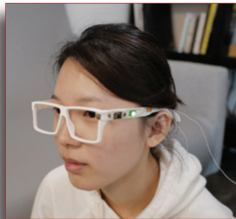
An MIT team used MorphSensor to design multiple applications, including a pair of glasses that monitor light absorption to protect eye health.
