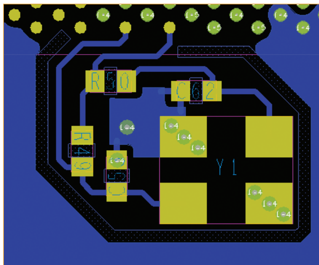
FIGURE 3. A crystal and its passive parts.
