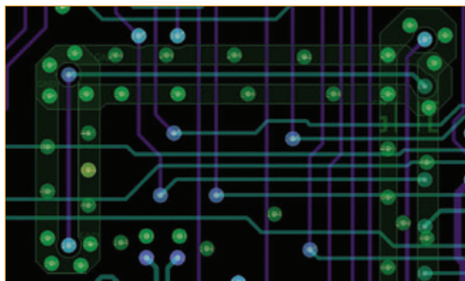
FIGURE 4. Guard bands around noisy traces. The surrounding low-speed signals benefit from the isolation.
