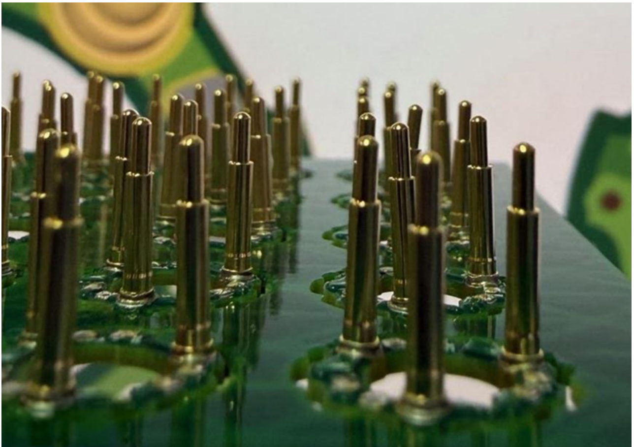
Figure 1. SMT pogo pins after reflow soldering, showing angular displacement beyond the customer's \pm 0.1^\circ tolerance from the required 90^\circ orientation.
