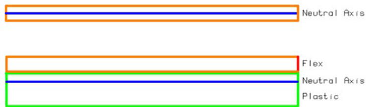
Figure 1. Bonding a flex circuit to a mechanical support shifts the neutral bend axis into the support material, increasing mechanical stress on the flex during dynamic bending.
