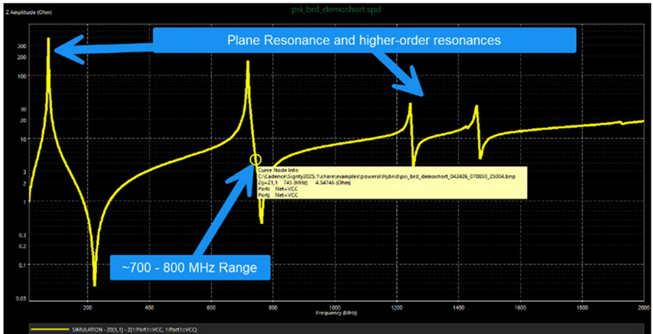
Figure 2. PDN impedance vs. frequency showing multiple cavity resonances. These peaks are driven by plane dimensions, dielectric spacing, and via distribution. Not regulator performance.
