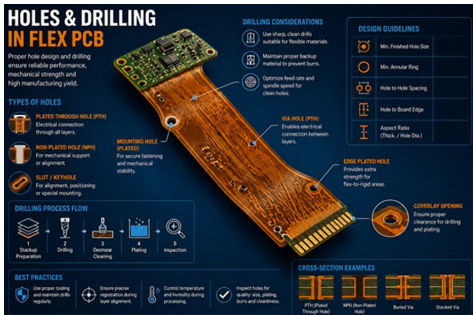
Figure 1. Flexible circuit fabrication is similar to the process for manufacturing rigid PCBs, but with a few key differences.
