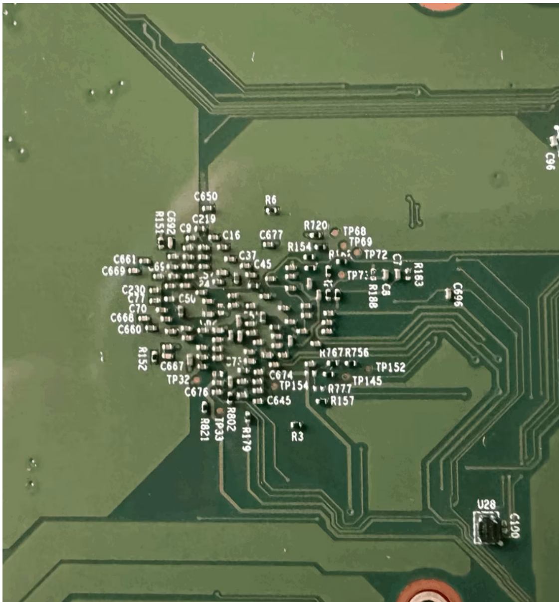
Figure 4. A cluster of 0201(imperial) caps and resistors plus a few test points support a processor on the opposite side of the board. Silkscreen was omitted from many of the components as there wasn't sufficient room.
