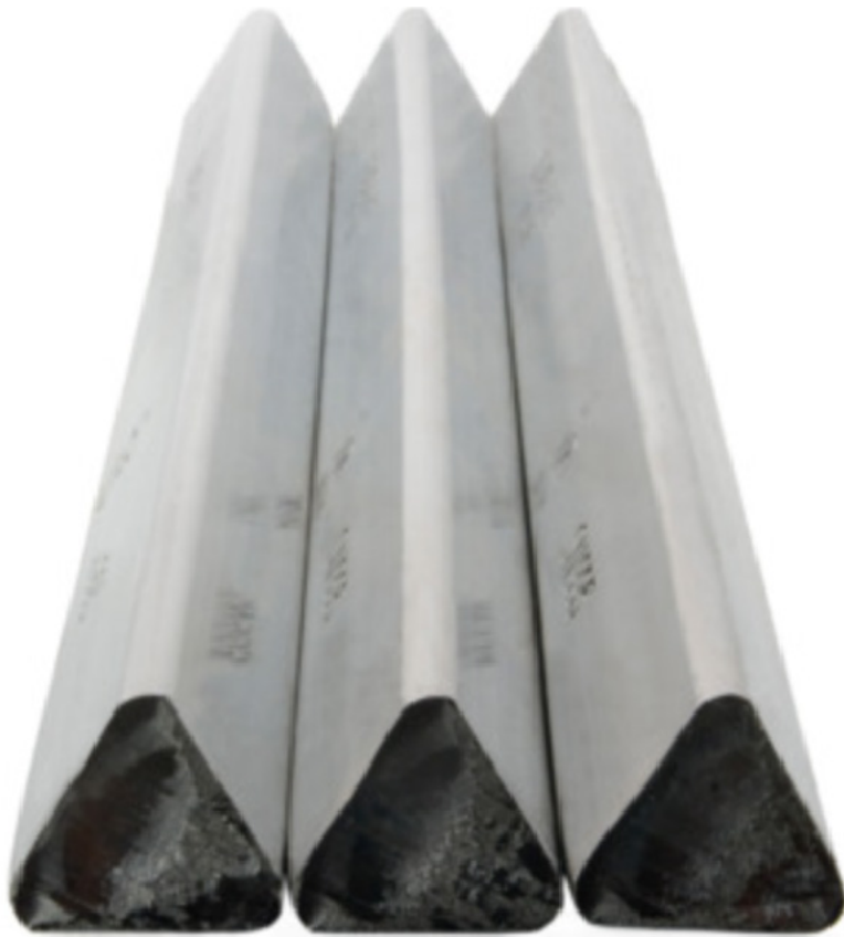
Figure 3. Bar solder was used in soldering for the telegraph industry starting in the mid-1800s.
