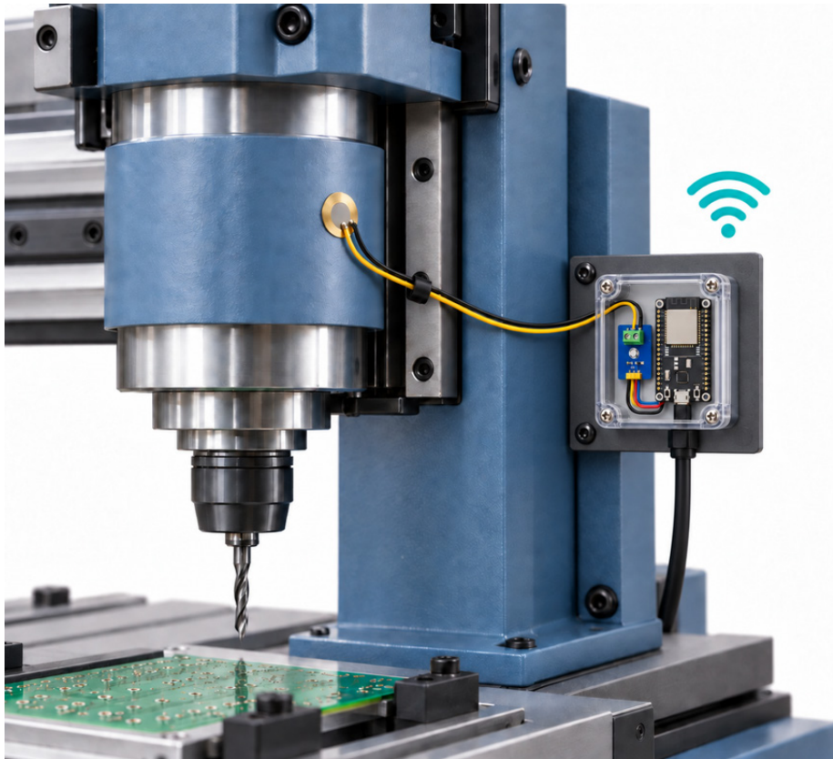
Figure 1. Low-cost sensors and small computers can give PCB fabricators greater visibility into equipment operation without replacing legacy machinery.
