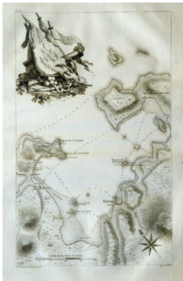
Lot. 3797 ..... Starting Price: 65 € Kauffer F., "Plan du port de Naoussa", Paris, 1782. This copper engraved map (37x25cm in a sheet 50x33cm) of the port of Naoussa on the island of Paros, is a very special map. It is the first map prepared with triangulation measurements in Greece. Choiseul Gouffier along with Kauffer, a skilled cartographer of the "Ponts et Chaussees", visited Paros in early 1776. The port of Naoussa was the main naval base of the Russian fleet in the Aegean (evacuated few months before the arrival of the team, in late 1775) and the French had strong interest in accurately map the naval base. Although the first partial triangulation has been done in Greece by Chambert in 1741 in Milos, this one is the first map of Greece of the modern time. An important map for the history of the Greek Cartography. Zacharakis 941/614
