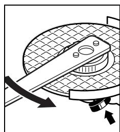
A properly fastened, undamaged quick-clamping nut can be manually loosened by turning the knurled ring in an anticlockwise direction.
