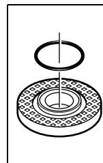
**Mounting flange for grinding spindle M 14:** A plastic part (O-ring) is fitted around the centring collar of mounting flange **10**. If the O-ring is missing or damaged, the mounting flange **10** must be replaced before resuming operation.
