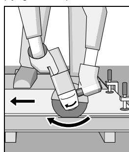
The machine must always work in an up-grinding motion. Otherwise, the danger exists of it being pushed uncontrollably out of the cut.
