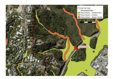
Figure 1: Flood mapping included in the Plan showing actual location of storm event
