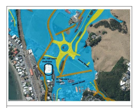
Figure 13: Flood Hazard Mapping in the Plan indicating modelled stream corridors, overland flowpaths and inundation for 100 year including Climate Change
