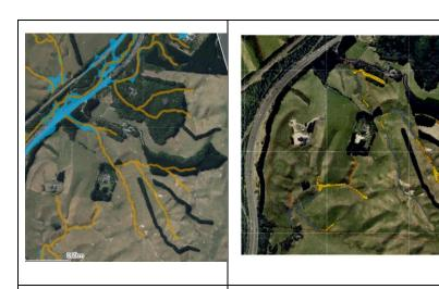
Figure 9: Flood Hazard Mapping in the Plan indicating modelled stream corridors
