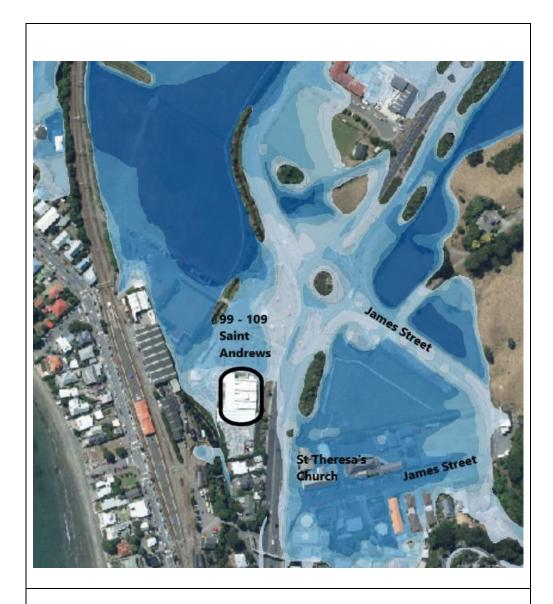
Figure 12: Flood Depth Mapping indicating modelled flood depths for 100-year including Climate Change
