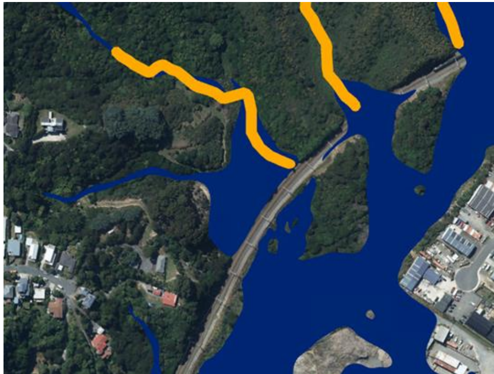
Figure 2: Updated flood modelling in response to the submission from Paul and Julia Botha [118.12] (yellow is Flood Hazard - Stream Corridor, and blue is Flood Hazard - Ponding)
