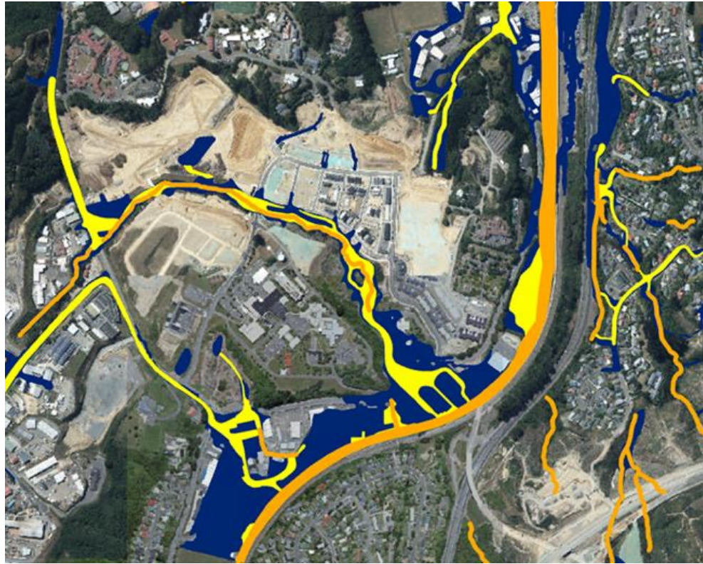
Figure 3: Updated flood modelling in response to the submission from Kenepuru Limited Partnership [59.29, 59.30] (yellow is Flood Hazard - Stream Corridor, and blue is Flood Hazard - Ponding)
