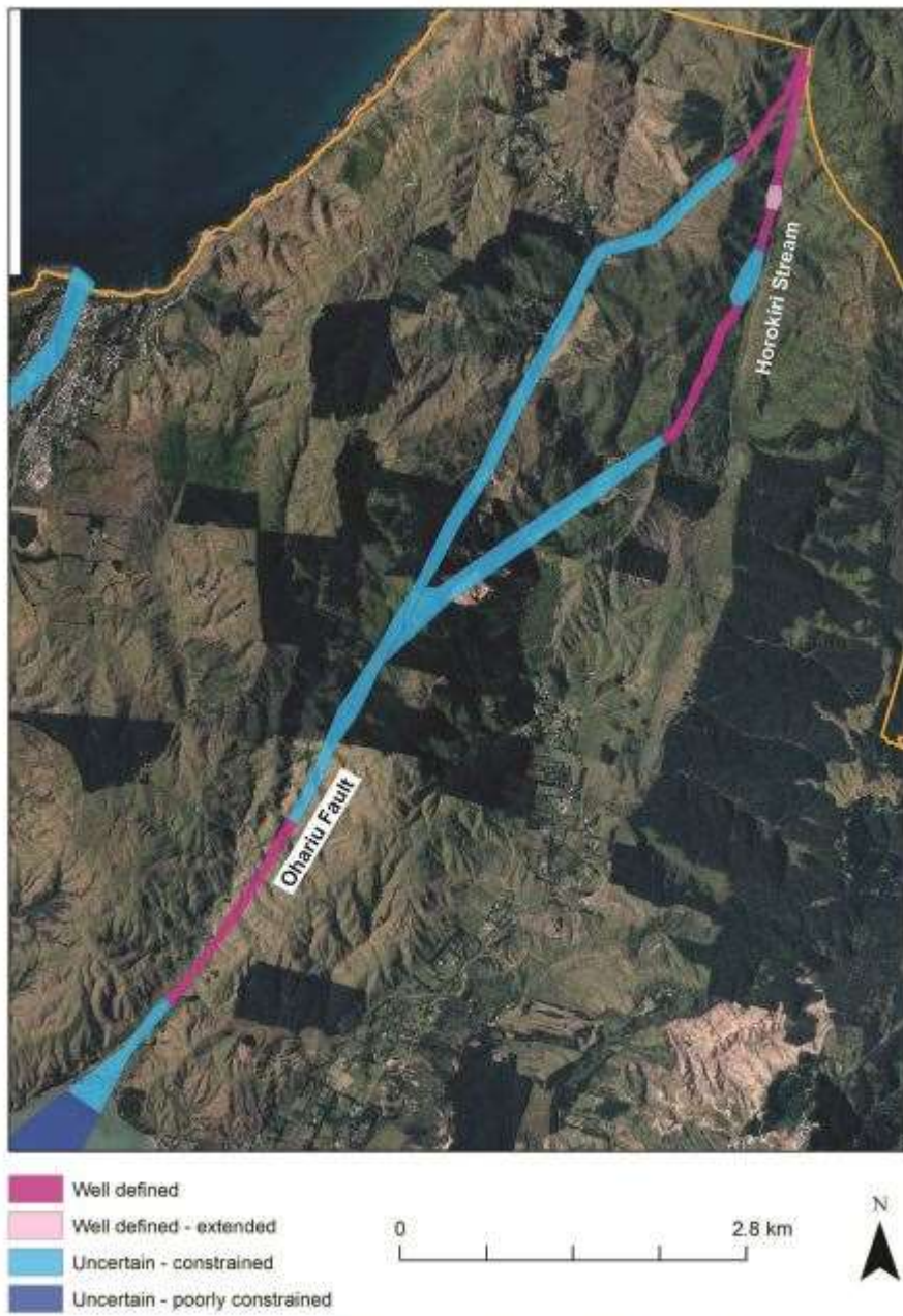
Figure 3 Fault Avoidance Zones for the northern half of the Ohariu Fault in Portrua District.
