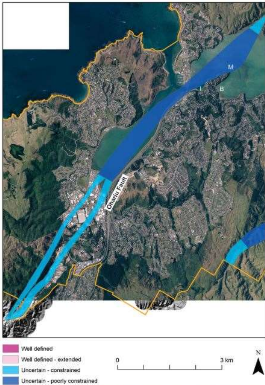
Figure 2 Fault Avoidance Zones for the southern half of the Ohariu Fault in Porirua District. B is Brown's Bay, I is Ivey Bay and M is Moorehouse Point.
