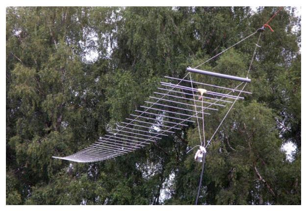
**Above**: a 47-element rope Yagi for the 144 MHz band, the elements (metal tubes) are 6mm diameter. In another design, rods of only 3.2mm diameter were used. The longest element is 1.05 metres, but the assembly length is 30 metres. The two ropes need only be 3mm thick.
