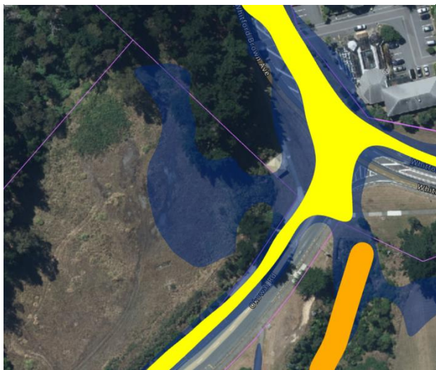
Figure 2 Current flood hazard mapping
