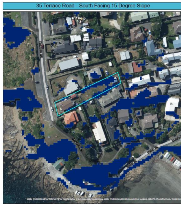
Figure 2: Plan with solid blue indicating south-facing 15 degree slope (from PCC's GIS database)
