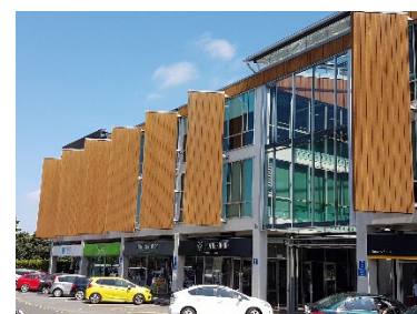
Subdivision and modelling of form and façade to reduce the apparent visual bulk of a building
