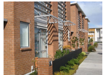
Projection of window bays, stepping of forms and gaps between units contribute visual interest to a terraced development. These images also show the value of frontage planting in adding to the visual richness and street appeal of the units.
