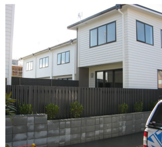
Rear yard given privacy by a combination of partial enclosure of that portion closest to the living room and low fencing and level change at the street edge.
