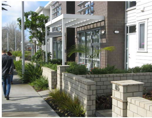
A sunny north-facing outdoor living area at the street edge, defined by a pergola and given privacy by planting and low walls
