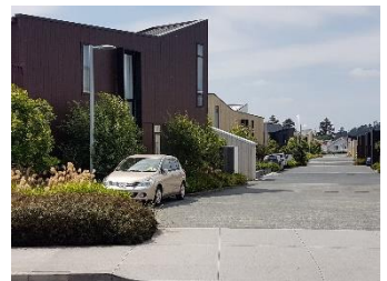
Shared surface rear access lanes which incorporate planting and subtle variation in paving and are overlooked from the houses served
