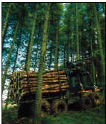
Used in conjunction with adequate brash mats, custom-built forwarders offer a site-friendly method of extracting thinnings from the forest.
