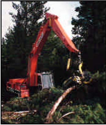
Some excavators can be fitted with harvesting heads and used as harvesting machines.
