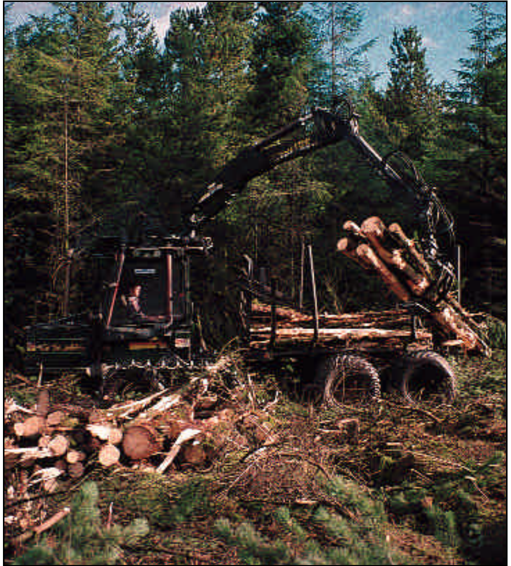
Forwarding is the most common method of clearfell extraction used in Ireland.
