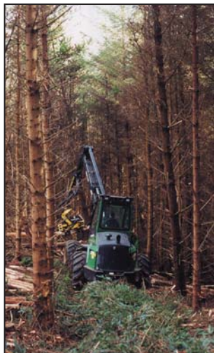
Opening the canopy may increase wind turbulence and allow the trees more room to sway. Brush mats protect the roots and soil. (Photo: S. Meyen)
