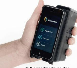
The Biomeme system includes a docking station for real-time qPCR, a mobile app to control the system and analyze results, and targeted test kits for preparing samples and identifying pathogens or diseases by their specific DNA or RNA signatures.
