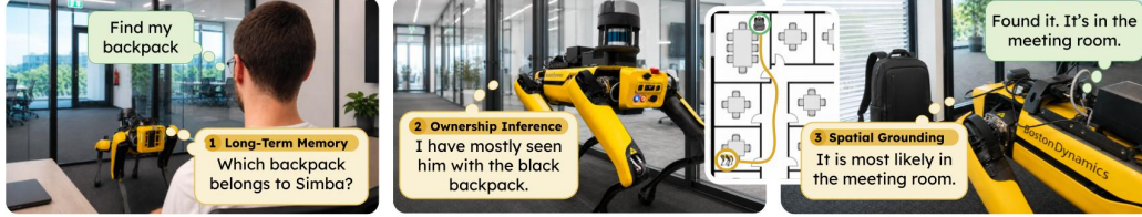
Figure 1: COOL enables personalized object search by combining long-term memory, ownership inference, and spatial grounding. Given a natural-language request such as “Find my backpack” (left), the robot first retrieves prior observations linking people and object instances, then infers the likely owner from accumulated human–object interaction evidence (middle), and finally grounds the selected object in the map to navigate to its most likely location (right).
