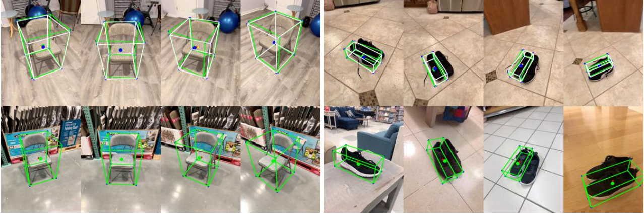
Figure 4. Examples of pose estimation for chairs (left) and shoes (right): our method enables us to obtain similar bounding boxes for pose estimation for each query frame. Furthermore, the fetched nearest neighbors also show similar attributes (e.g. shape) compared to the query frames. The ground truth and obtained 3D bounding boxes are shown as yellow line overlays.
