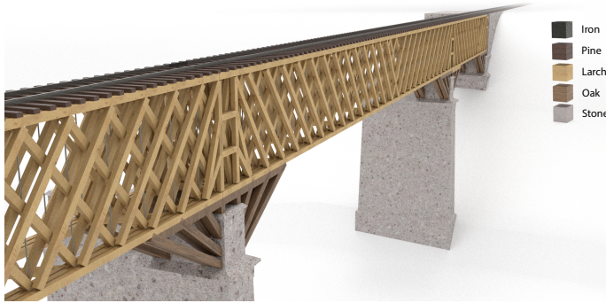
Fig. 11. Illustration of the main element of the King Louis Bridge : Between the two stone pillars (light gray), the bridge has been made almost entirely of wood (light brown for larch and dark brown for oak) as it is cheap and can absorb compressive forces well. However, wood does not tolerate tensile forces well, especially at the joints for which reason Howe used round iron rods (dark gray) for the vertical struts of the truss bridge, which were tensioned with screw nuts. As illustrated here, the diagonal compression struts were still made of wood. The railroad ties have been modeled from pine wood (wenge) and the tracks have been made out of iron (dark gray). The element shown here is 52 m long.
