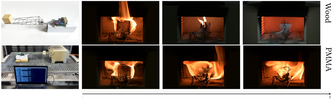
Fig. 7. Experimental setup for mass loss and temperature measurement. Samples of different materials (wood and PMMA) are equipped with thermo probes and placed on a scale arm inside an oven that heats the sample up until the ignition temperature. During the combustion process, the weight and temperature and different depths (surface, sub-surface, and core) are continuously recorded.
