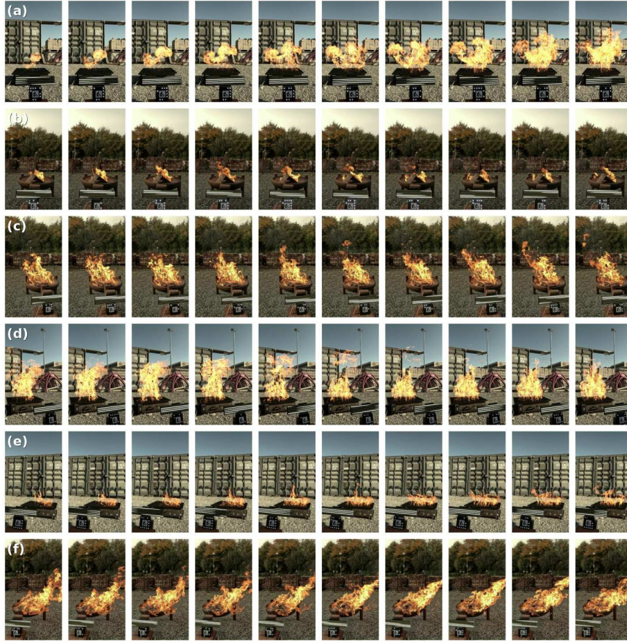
Fig. 4: Qualitative overview of our real-world fire dataset. Sequences (a,d,e) depict a propane jet of varying intensity, (b) is comprised of wooden logs, (c) are sheets of cardboard, and (f) is a pile of crumpled paper. Each scene progresses temporally from left to right.
