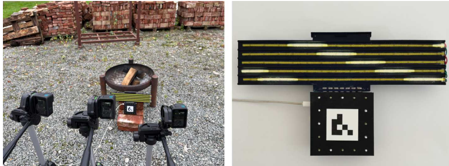
Fig. 3: Real-world capturing setup. The left image depicts the camera and fire setup, while the right image shows the custom hardware used for visual synchronization of the cameras. The partially lit LEDs within its top section clearly depict the rolling shutter effect used for sub-frame synchronization.
