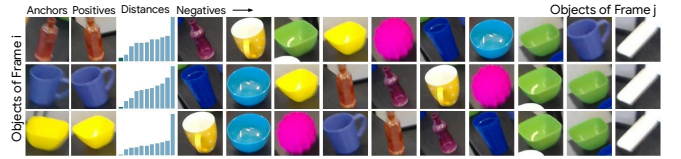
Fig. 3. View-to-view object correspondences: the first column shows all objects detected in one frame (anchors). Each object is associated to the objects found in the other frame, objects in the second column are the nearest neighbors (positives). The third column shows the embedding space distance of objects. The remaining objects (negatives) are shown from left to right in descending order according to their distances to the anchor (not all objects shown).
