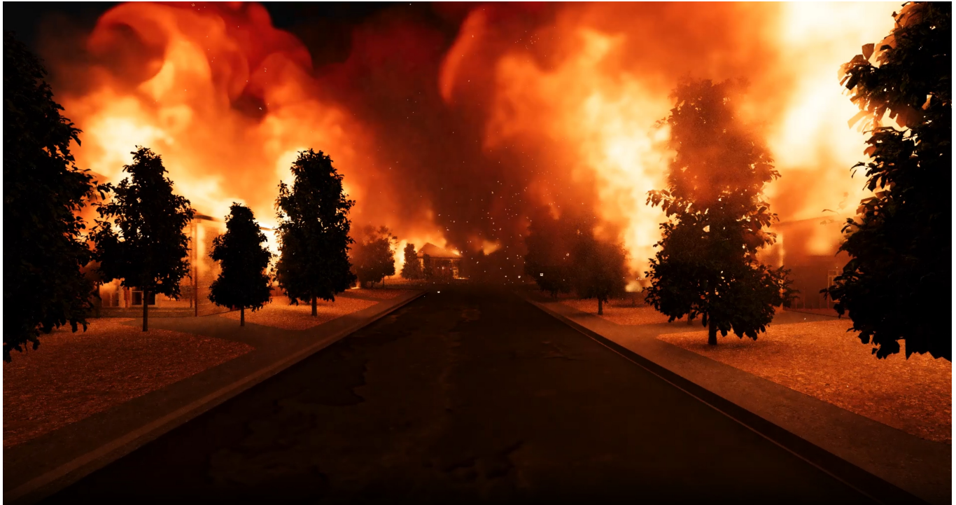
Fig. 1. An urban wildfire simulated with our framework: by leveraging a fuel-centric representation for modeling the environment, our method allows us to simulate the combustion of vegetation and buildings, while considering several fire propagation mechanisms.
