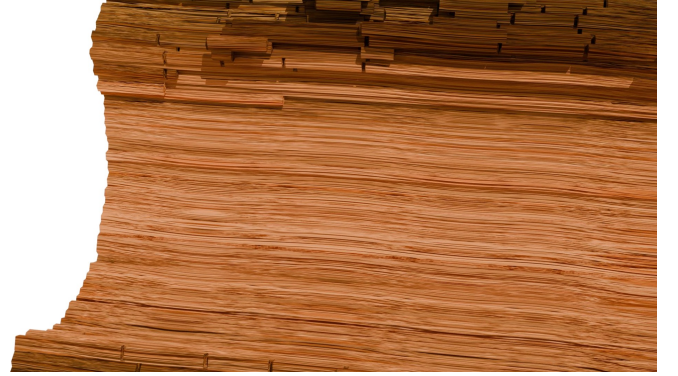
Fig. 8. Lignin-degrading decay yields a smoother, more diffuse weakening pattern than brown rot: material loss spreads gradually through the volume, producing softened, stringy wood with an irregular surface rather than blocky fracturing.
