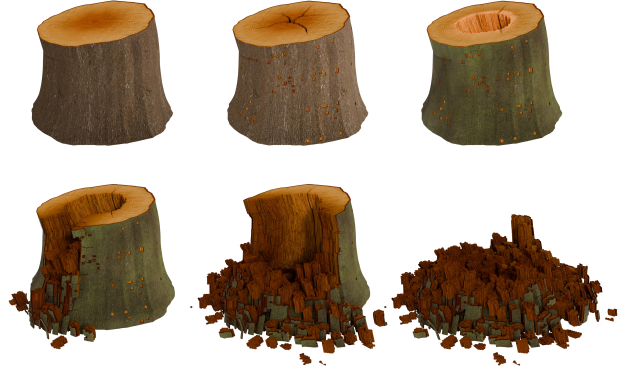
Fig. 14. Evolution of wood decay of a cut tree trunk (top, left): Internal cracks emerge because of the moisture change (top, middle). The heartwood's low resistance makes it vulnerable to white rot, causing it to become hollow (top, right). Due to brown rot, the wood decays further (bottom, left) until it is fully affected by rot (bottom, center), and then it further decomposes (bottom, right).
