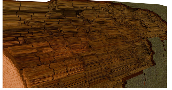
Fig. 7. Close-up of brown rot fungal decay in wood, highlighting the characteristic cuboid fracturing pattern caused by the fungus, leaving the wood dry, brittle, and cracked into distinct blocky segments.
