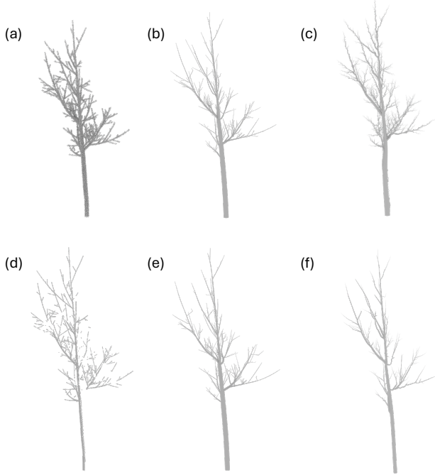
Fig. 17. Comparison with QSM on different LiDAR scanning data. (a) and (d) show the same tree scanned by full sampling and TLS simulation. Compared with QSM results (c) and (f), our model can generate more realistic tree shapes with fewer twisting artifacts.
