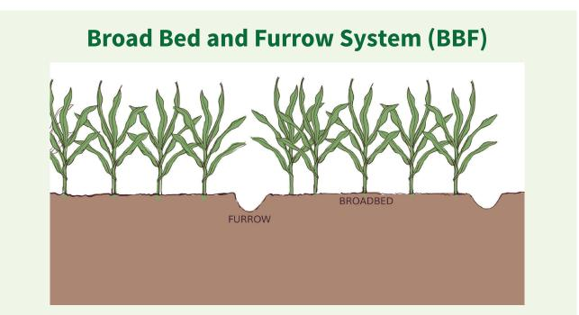
In a broad bed-and-furrow system, runoff water is diverted into field furrows (30 cm wide and 30 cm deep). The field furrows are blocked at the lower end. When one furrow is full, the water backs up into the head furrow and flows into the next field furrow. Between the field furrows are broad beds about 170 cm wide, where crops are grown.
