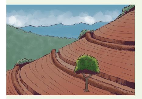
These are 2 by 1 by 1 m3 and 5 to 10 feet vertical distance. trenches that are excavated in contours and excavated soil is used to form bunds in the down line. They are suitable where the slope of land is greater than 33.33%., which helps to reduce the velocity of water as well as soil erosion.
