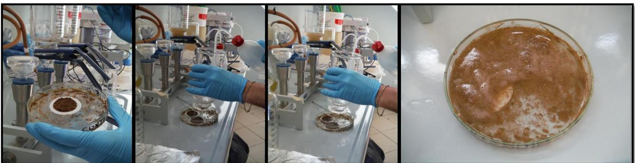
Figure 3. Representation of the filtration apparatus positioned into the hood, to prevent environmental contamination of MPs. Main steps of the extraction method include filtration of the supernatant, recovery of the membrane and overnight digestion of organic material in 15 % H<sub>2</sub>O<sub>2</sub>.
