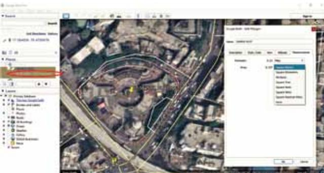
Figure 2.12: Area measurement and accounting after main plot demarcation
