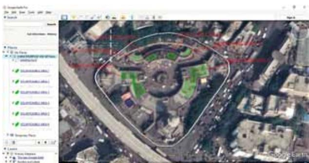
Figure 2.15: Solar feasible areas under green polygons
