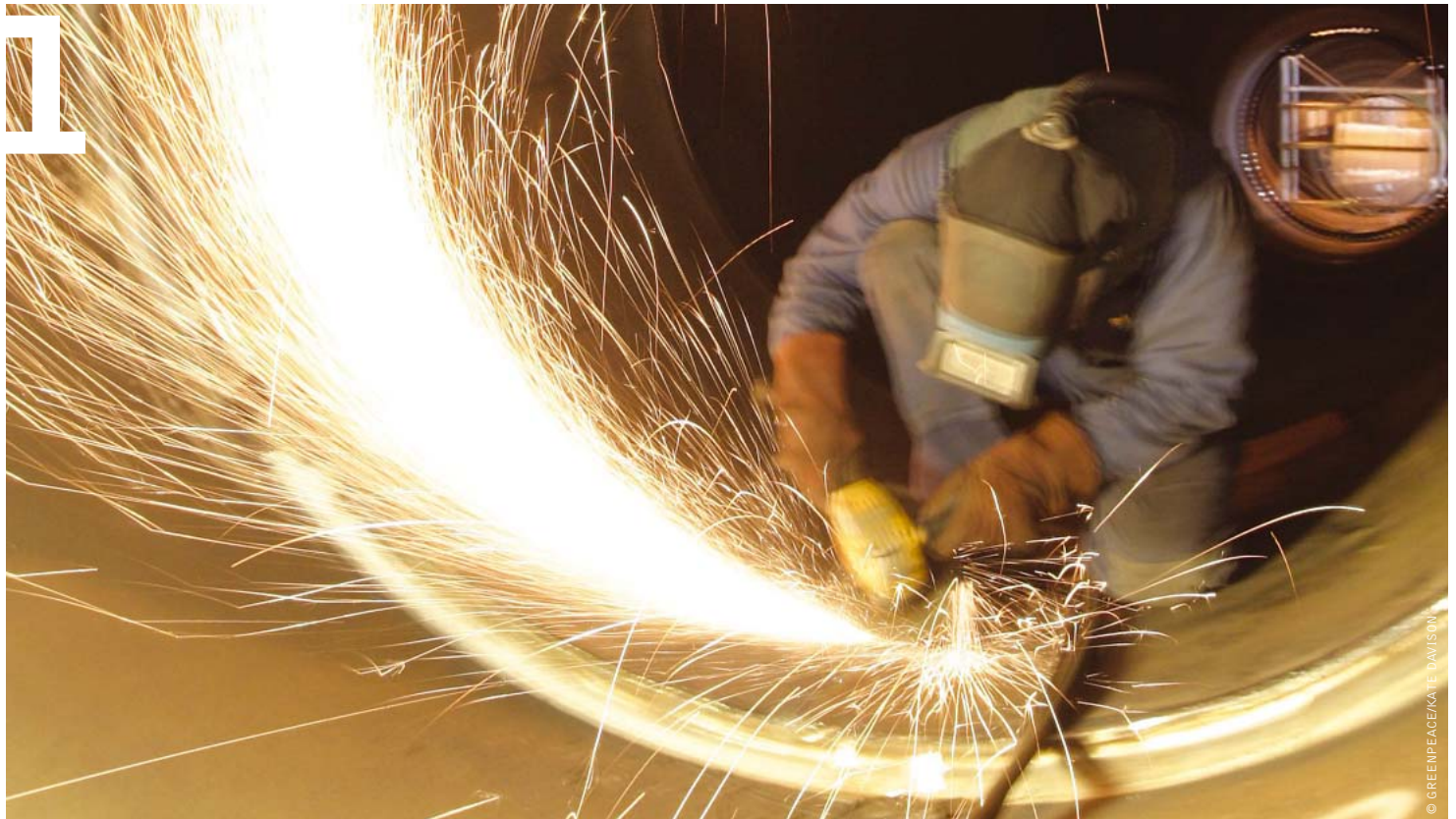
image MAN USING METAL GRINDER ON PART OF A WIND TURBINE MAST IN THE VESTAS FACTORY, CAMPBELLTOWN, SCOTLAND, GREAT BRITAIN. WIND TURBINES ARE NOT ONLY A SOURCE OF RENEWABLE ENERGY, BUT ALSO OF EMPLOYMENT.
