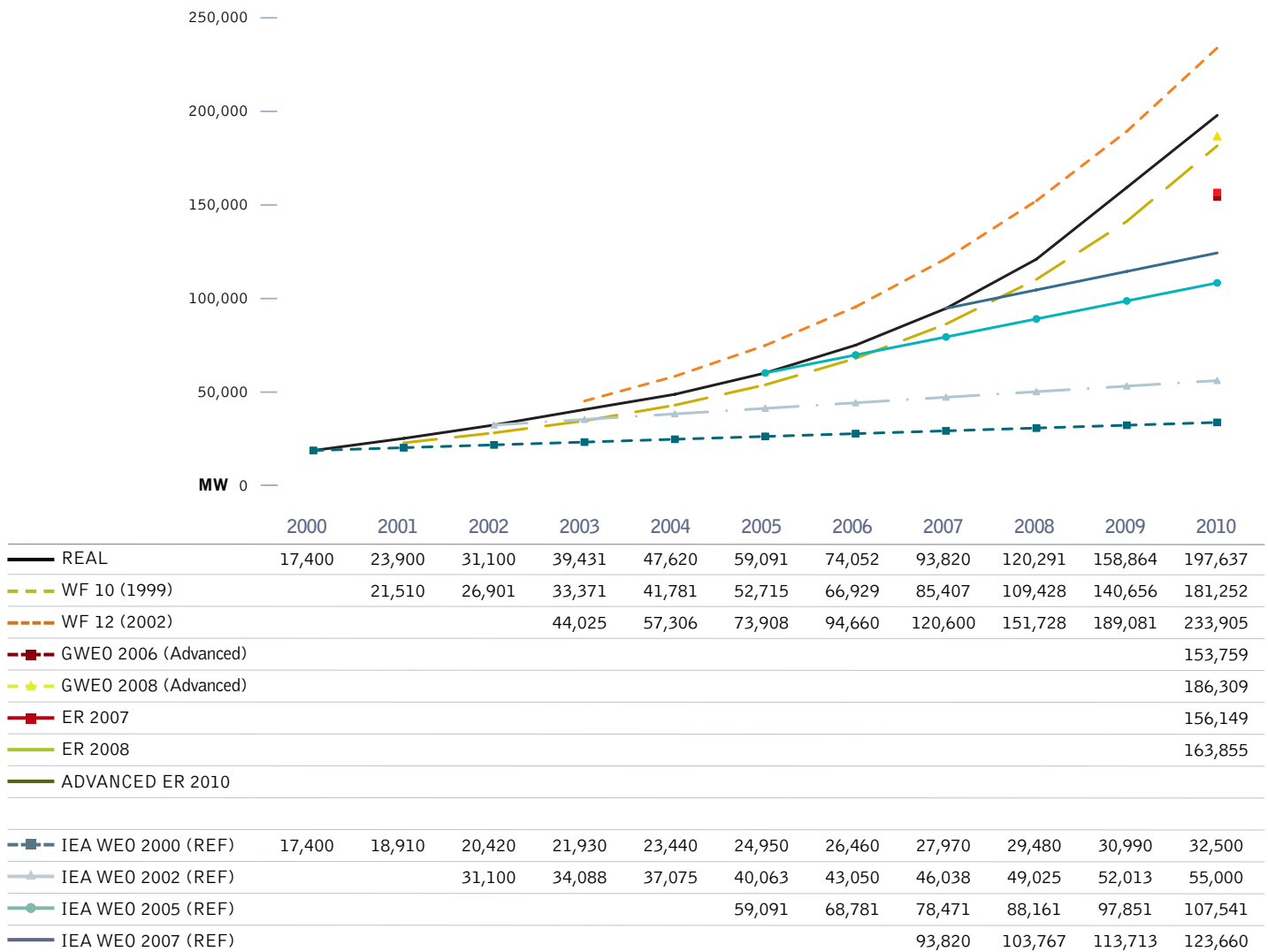
figure 4.5: wind power: short term prognosis vs real market development - global cumulative capacity
