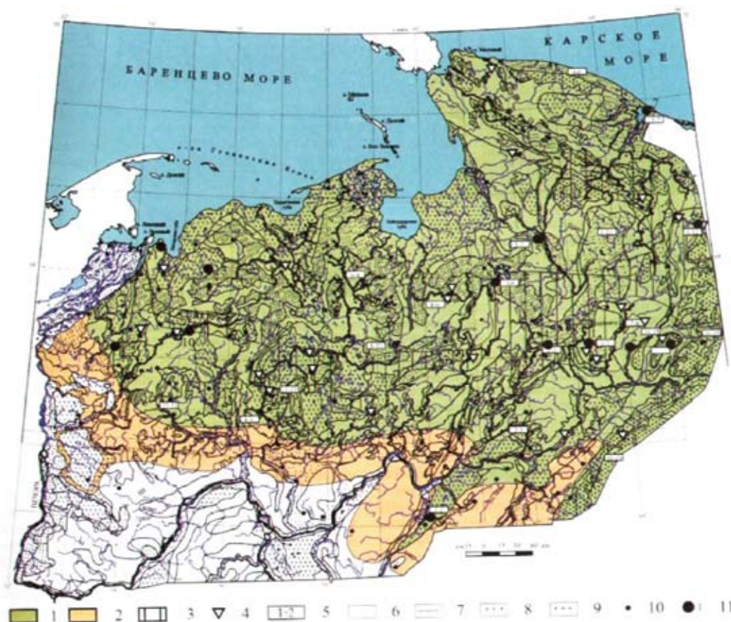
Fig. 3. Permafrost dynamics of the ETP North for 1970-2005 r. 1 – distribution area, as per 2005, 2 – a part of sporadic permafrost zone thawed wholly or partially during 1970-2005 r. 3 – a part of a zone of continuous permafrost distribution (as per 1970), which became a zone of discontinuous distribution by 2005, 4 – taliks whose thickness is more than 15 m, appearing within the studied period, 5 – deepening of taliks which existed before, 6-9 – different soil types: loam sands, peat, rocks, 11 – geocryological stations. (Oberman, Shesler, 2009).
