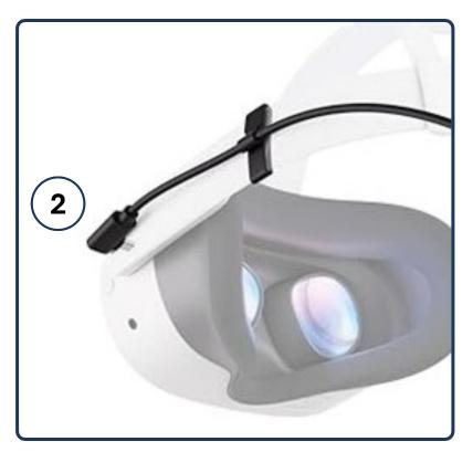
Connect the cable to both the PC 1 and the VR headset 2. Make sure the cable is firmly secured to prevent accidental disconnection.
