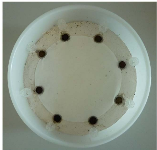
Figure 1. Experimental setup of the feeding chambers. Plastic boxes (diameter 18 cm, height 8 cm) filled with gypsum (4 cm) and eight microcentrifuge tubes containing litter material (one for each plant species, randomly placed). doi:10.1371/journal.pone.0045345.g001
