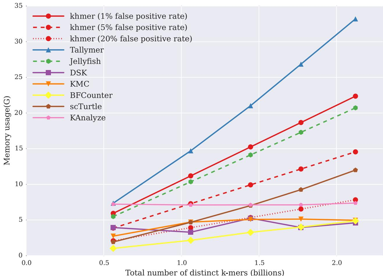
**Figure 2. Memory usage of k-mer counting tools when calculating k-mer abundance histograms, with maximum resident program size (y axis, in GB) plotted against the total number of distinct k-mers in the data set (x axis, billions of k-mers).**
