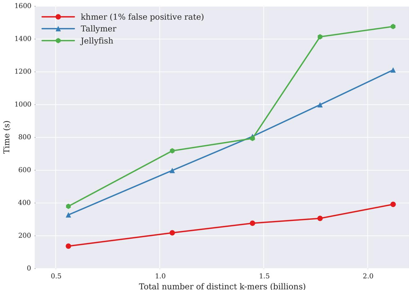
**Figure 4. Time for several k-mer counting tools to retrieve the counts of 9.7 m randomly chosen k-mers (y axis), plotted against the number of distinct k-mers in the data set being queried (x axis).** BFCOUNTER, DSK, Turtle, KANalyze, and KMC do not support this functionality. doi:10.1371/journal.pone.0101271.g004
