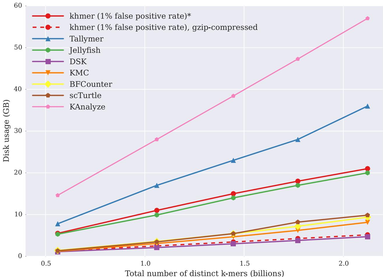
**Figure 3. Disk storage usage of different k-mer counting tools to calculate k-mer abundance histograms in GB (y axis), plotted against the number of distinct k-mers in the data set (x axis).** \*Note that khmer does not use the disk during counting or retrieval, although its hash tables can be saved for reuse.
