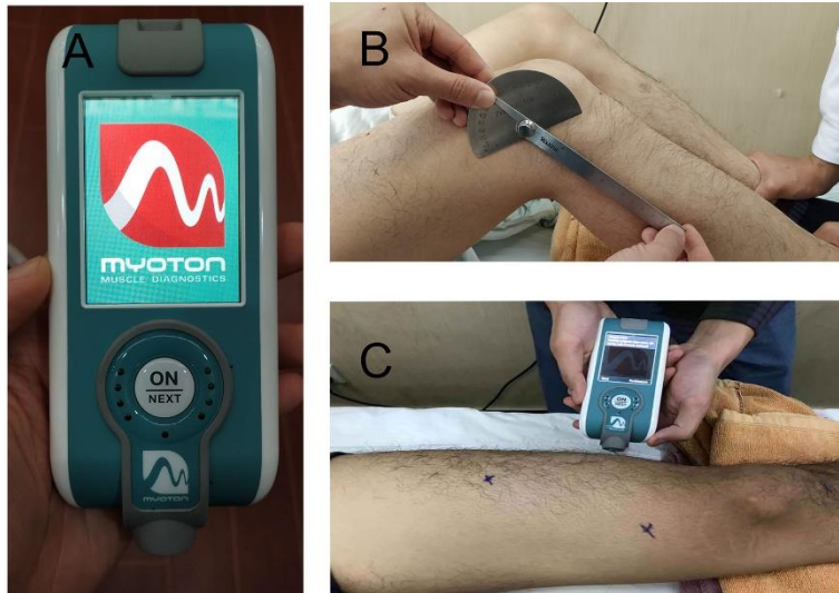
S1 Fig. The MyotonPRO measurement technique. (A) MyotonPRO device; (B) Identification of measurement angle; (C) Measurement with MyotonPRO.
