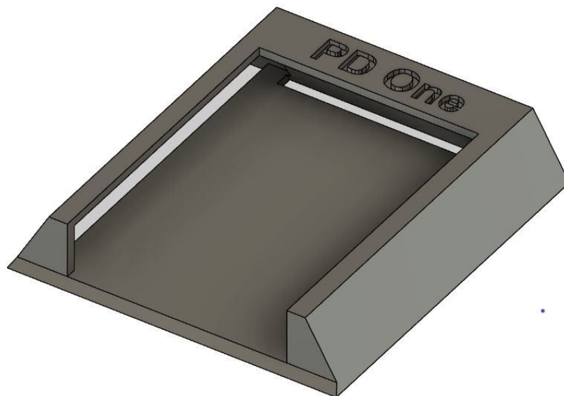
Fig. S06. Top of the box with side space with the inclination for the allocation of LEDs.
