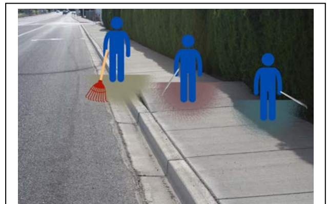
Fig. 26. A team of three using the snowplow method to observe the edge of the sidewalk to the edge of the gutter. Rake being used to remove debris from gutter and cracks in the paving.
