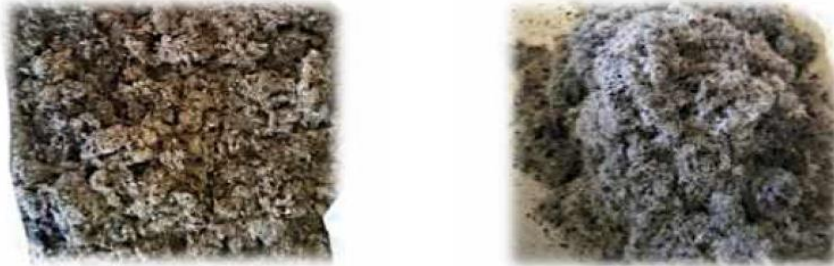
Fig. 2 Tyre polymer fibres before (left) and after (right) processing for reuse
