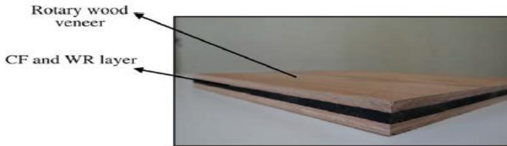
FIG. 2. Layers arrangement of the reinforced plywood panels.
