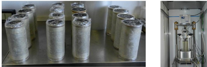
Figure 2. (a) Cylindrical Specimens Ø 100 mm H 200 mm (b) Cyclic Load Triaxial Test.
