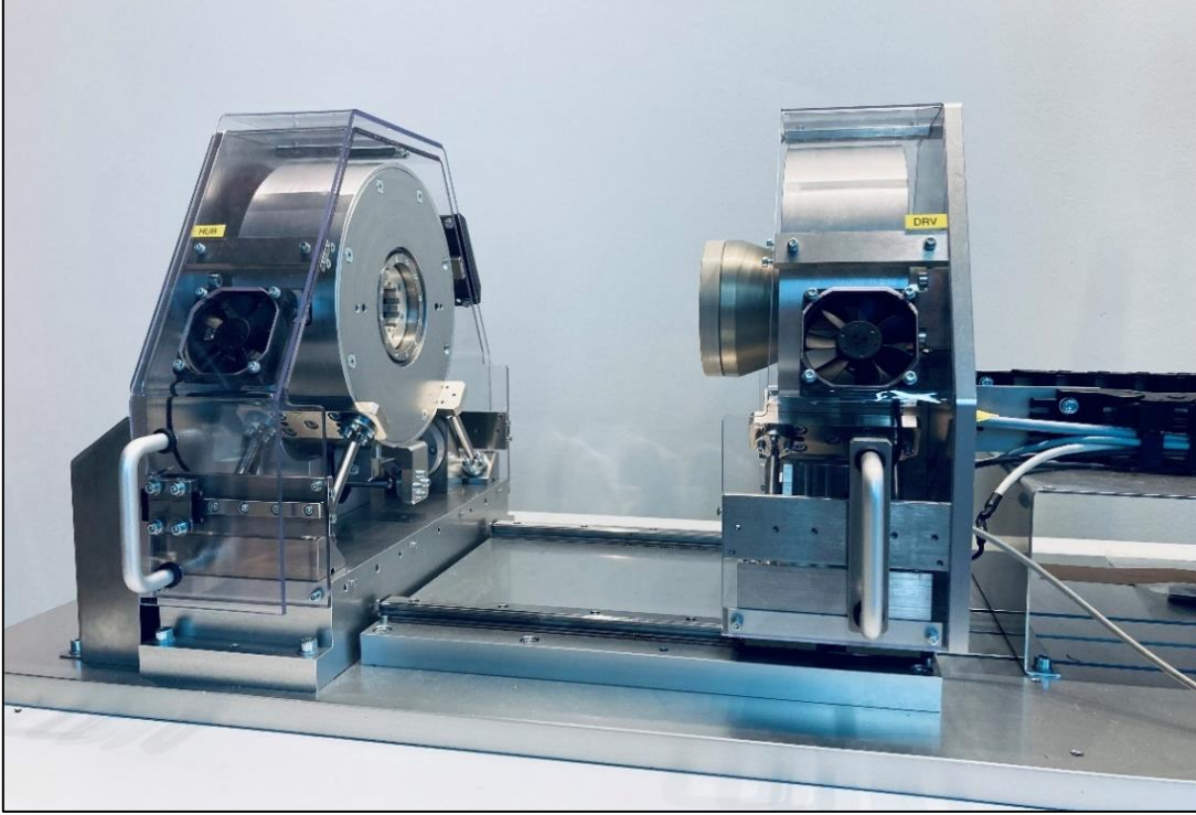
Figure 15. The efficiency test rig infrastructure in the isolated hub configuration
