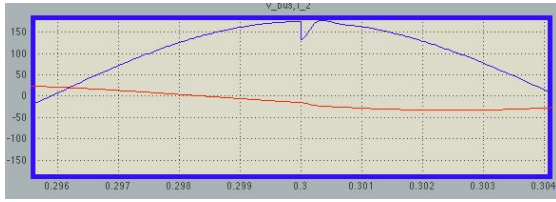
Fig. 3. The data shows how the local impedance controller manages substantial reactive loads, without Q compensator in the system.
