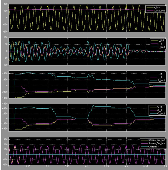
Fig. 4. Simulation trace showing synchronization and hot-connect at t = 0.03 seconds.
