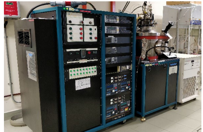
DC/RF Magnetron Sputtering(AJA) 4-Gun System
