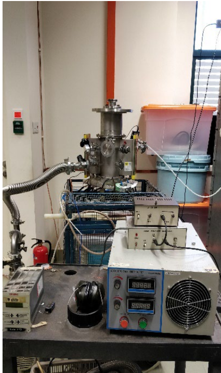
UNU-ICTP DPF Maximum Operating Voltage: 15kV Capacitor: 30 \mu F Energy: 3 kJ
