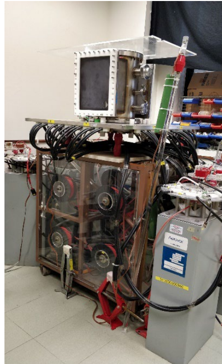
NX-3 DPF Maximum Operating Voltage: 20 kV Capacitor: 100 \mu F Energy: 20 kJ
