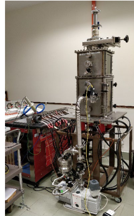
LVSMF DPF Maximum Operating Voltage: 13 kV Capacitor: 350 \mu F Energy: 40 kJ
