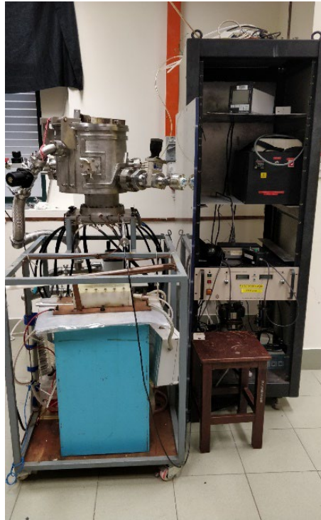
Carbon-ICTP DPF Maximum Operating Voltage: 15kV Capacitor: 30 \mu F Energy: 3 kJ
