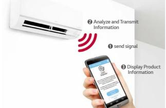
\* When the model doesn't provide embedded Wi-Fi, diagnose by buzzer sound with the same app and remote controller
