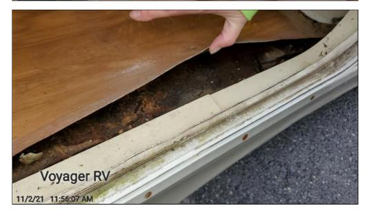
(2) Observed deteriorated seals on rear cargo door and evidence of water intrusion inside cargo area. Recommend repair by a qualified RV technician to prevent future water intrusion.
