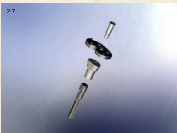
Illustration: Modular Shaft combined with the Modular Sleeve Component on the BCK Tibial Tray
