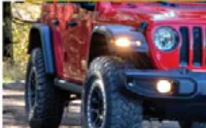
Flat Design Offers Additional Clearance for Tires
