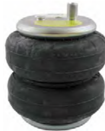
ULTRR6397 Air inlet: 1/8 NPT Ride Height: 5.50"-6.50" Max. Diameter: 6.6" For: ULTRR2350
