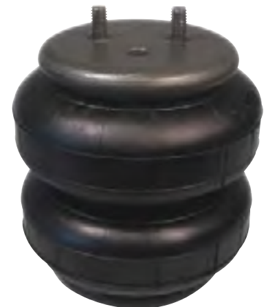
ULTRR6781 Air inlet: 1/4 NPT Ride Height: 5.50"-6.50" Max. Dia.: 6.60" For : ULTRR2071
