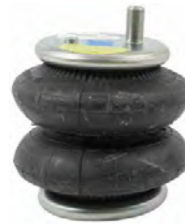
ULTRR6401 Air inlet: 1/4 NPT Combo stud: 3/4" - 16 Ride Height: 5.50"-7.00" Max. Dia.: 7.52"
