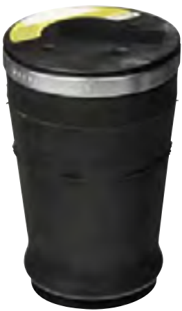
ULTRR9002 Air inlet: 1/4 NPT Ride Height: 7.25" Max. Dia.: 6.60" CHEVROLET / GMC 88-98 Silverado/Sierra 1500 2WD only DODGE 97-03 Dakota 4WD only not Crew Cab 97-02 Durango 2WD/4WD not SXT 94-01 Ram 1500 2WD only 03-06 Sprinter 2500 2WD only FORD 98-14 E250
