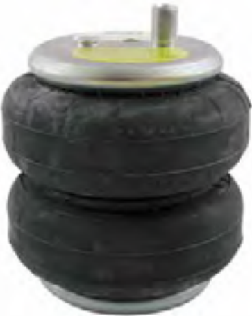
ULTRR6397 Air inlet: 1/8 NPT Ride Height: 5.50"-6.50" Max. Diameter: 6.6" For: ULTRR2350
