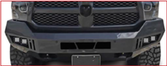
PRODUCT CODE: ULTFLDB008TI Bumper; TFX Front LD Bumpers; One Piece Design; Direct Fit; Mounting Hardware Included; Without Grille Guard; Without Winch Mount; Without D-Ring Mount; With 3 Inch LED Cube Light Cutouts And 20 Inch Double Row Straight Light Bar Cutout; Black Titanium Powder Coated Steel • With Sensor Holes - OE Sensor Compatible
