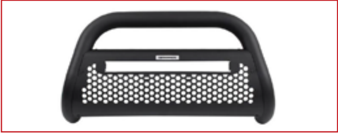
PRODUCT CODE: ULT55663T Bull Bar; Charger- RC2 Light Ready; Black Textured Powder Coated Mild Steel; 3 Inch Diameter; With 20 Inch Central Light Mount; With Hexagonal Mesh Skid Plate; Without Light Bar Installation Will Interfere With Parking Sensors, Proximity Sensors, Forward Facing Laser Brake, Camera, Lane Keep Assist, and Cruise Control Sensors
